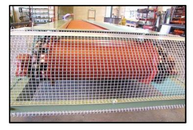
composed of articulated plates, made of structural steel fixed to special roller chains for heavy transport with hardened pins, bushes and cemented rollers. Tensioning is carried out by means of double screws acting on the return axis. The planetary gearboxes are directly keyed onto the drive shaft and coupled to self-braking flanged electric motors. The 8 tooth crowns are fitted with BIKON system locking sets. The quality steel shafts are mounted on roller bearings in heavy series bearings.
