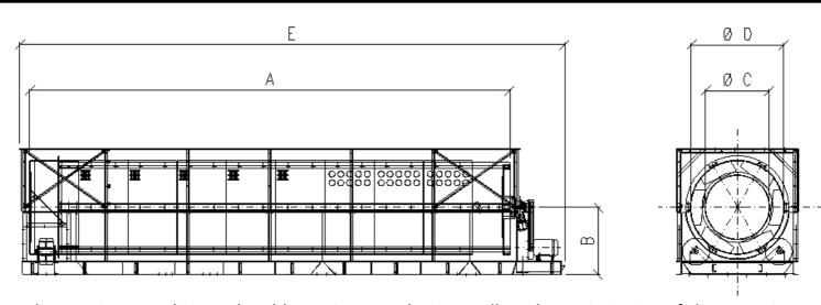
The rotation speed is regulated by an inverter device to allow the optimization of the screening yield as the input load varies. The transmission system is made using a planetary gearbox for cement mixers. The rear support wheels (load side) are in heavy duty solid rubber. The conveyor belts applied to the screens are dimensioned with abundance to avoid any possible clogging; they are also particularly robust in order to accept the large and heavy parts bypassed by normal shredders.
